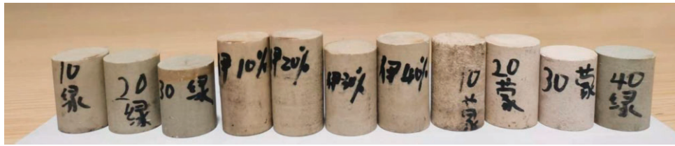
Figure 3. Different clay-bearing sandstone samples at the compression pressure of 15 MPa.
